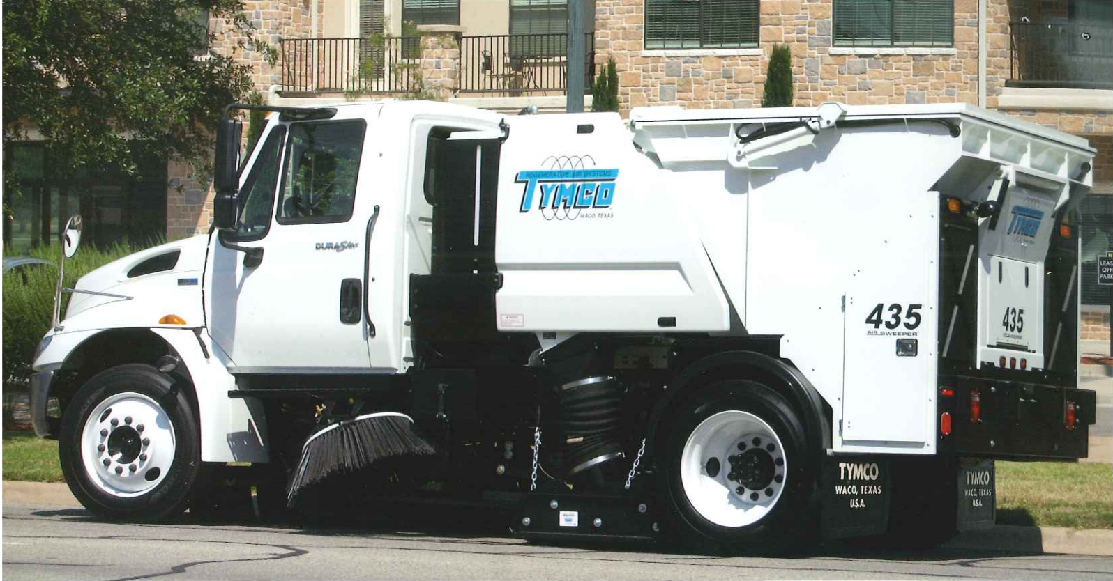
The Model 435 delivers street sweeping performance in a mid-sized package. With the Conventional Truck Package, the Model 435 has a payload of over 8000 lbs. and overall sweeping path of 132 inches.
