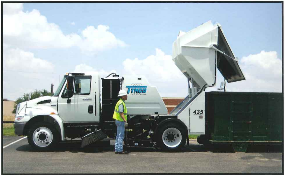
With the Conventional Truck Package, the Model 435 has a 81 inch dump height. (Most 30 yard containers are approximately 69 inches)
